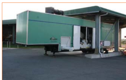
Figure 4. Trailer-mounted Cyclonic Thermal Dryer.
